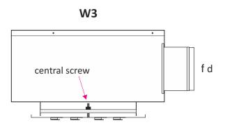
Central assembly through the crossbar (WMC) mounted in the plenum box and the central mounting screw.
